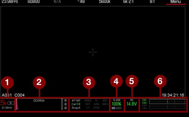
The bottom row is referred to as the Lower status Row. It provides access to key system information and camera values (from left to right)
